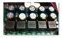
Traditional I-shaped inductors, toroidal inductors and chip inductors have improved the efficiency of digital power amplifiers. The new type inductor uses Mn-zn ferrite material and special structure, which has excellent shielding effect and working efficiency. In addition, its linearity is better than that of a toroidal inductor in terms of
